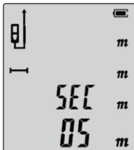
Now use the "-" and "+" - buttons to set the seconds to the time-delayed measurement and confirm by pressing the "ON/MEAS" key (1). Now begins a countdown to zero, in which the measurement is initiated
