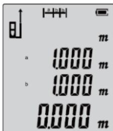
Change the value of the distance (a) with the "-" and "+" - keys and confirm the value with the "ON/MEAS" key (1). Now change the value for the flashing second distance (b) also with the keys "-" and "+". Confirm again with "ON/MEAS" key (1).
