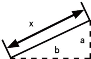
Measure to the first cathetus ( $a$ ) with the "ON/MEAS" key (1). Then flashes the second cathetus ( $b$ ) that you measure with the "ON/MEAS" key (1). In the main line now the result of the hypotenuse ( $x$ ) is displayed.
