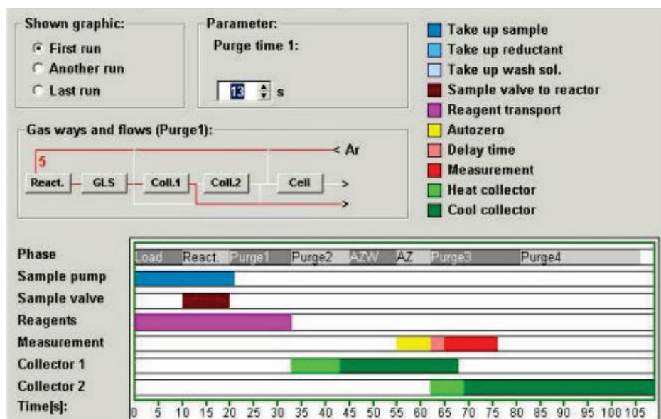
Fig. 5-19 Measurement with Enrichment and Transfer, Time Schematic Chart
