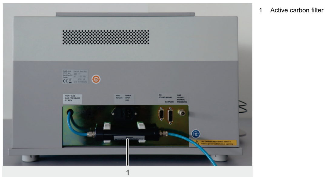
Fig. 5-10 Active Carbon Filter at Gas Inlet
