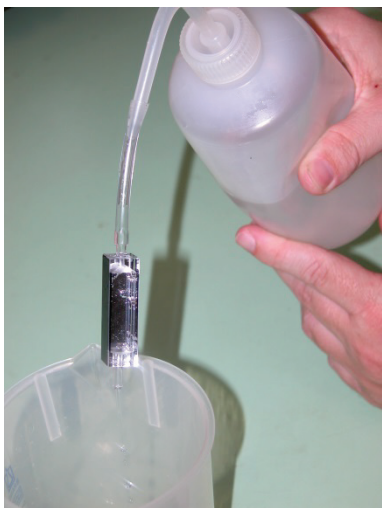
Cleaning of Cell
